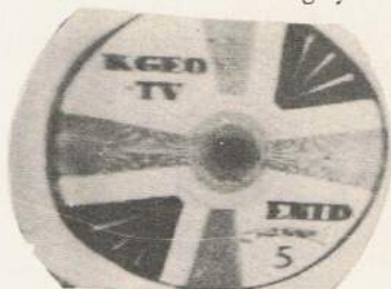
With the MUF riding 82 megs, KCEO-5, Enid Oklahoma, seen in Fresno, Calif. (Cooper) a good grade Es signal.
