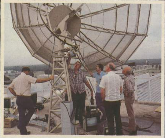
NASA engineers watch Paradigm chief engineer Frank Casten (plaid shirt) and Paradigm engineer Gene Campbell fine tune the 4.8 meter with a spectrum analyzer.
