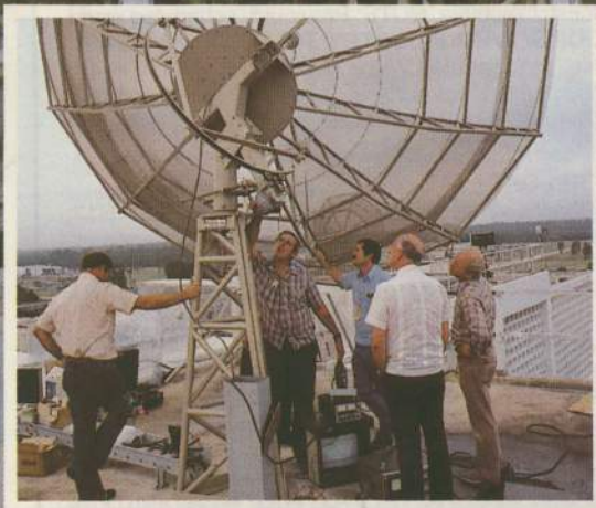
NASA engineers watch Paradigm chief engineer Frank Casten (plaid shirt) and Paradigm engineer Gene Campbell fine tune the 4.8 meter with a spectrum analyzer.
